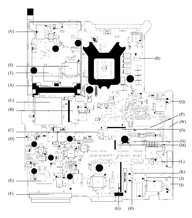
Figure B-1 System board (FMSSY\* 32M) layout (front)
